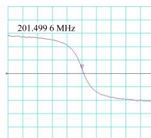
图2 RFQ 加速腔 S21 参数的相频曲线 Fig.2 Phase-frequency response curve of RFQ cavity.
